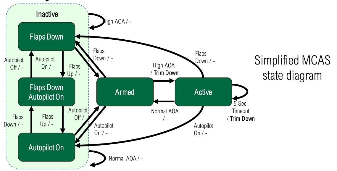
Using the Gherkin system test language, design a system test to verify that MCAS activates (that is, produces a trim-down input) as desired
